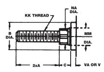
High Tensile, rolled thread stud with two times **A** length is available on Rods thru 2" in diameter.
