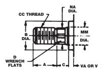
Male thread larger in diameter than style 2. No shoulder for locking. Stud not used.
