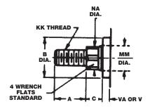
Male thread with adequate shoulder for locking accessory. High tensile, rolled thread stud used on all Rods thru  $2^{1}/2^{"}$  in diameter.
