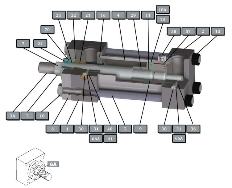
Round, single piece rod gland and retainer used on all but some of the smaller bore sizes. Consult pages on specific mounts.
