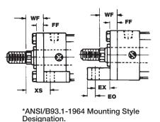
**IMPORTANT NOTICE** SL and CL MOUNTS - The round gland retainer shown above is not used on the  $1^{1}/8^{"}$  bore,  $1^{1}/2^{"}$  bore, or the  $2^{1}/2^{"}$  bore with a  $1^{3}/4^{"}$  rod diameter and the  $3^{1}/4^{"}$  bore with a  $2^{"}$  rod diameter
